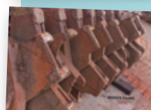
A cane knife mounted on rotor palms cuts cane for shredding
