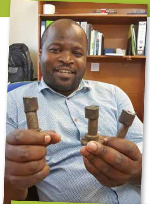
*"Preventative measures which entails highly technical procedures are now needed and equipment must be checked often. We do condition monitoring of the machines and also send oil samples away for tribology which will tell us what is wrong and needs to be corrected. At present we are also replacing all the worn-out bolts."*
